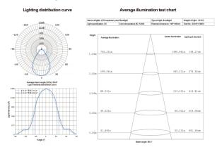
Notes: The photoelectric parameters are authentic data represented by the RLB 81 83 light of power 20W, for reference only
